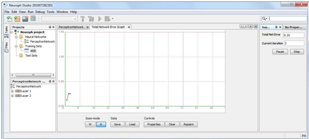
**Step 5.** After the training is complete, you can test the network for the whole training set by selecting training set to test, and clicking Test button..
